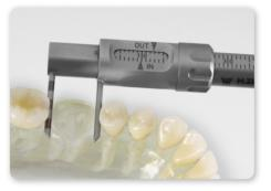
OUT shows the determined outside dimension (Ø 1.5 mm), IN shows the inner diameter.
